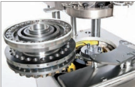
Fast exchange of die table
